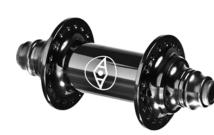
3/8" Bolt-On race front Details: Small flange, press fit system Body: 6061 T6 Axle: 7075 T6 15 mm hollow axle Bearing: Stainless sealed cartridge bearings Holes: 36 Colors: Black Pitch Center Diameter: 45 mm Center to Flange: 29 mm Weight: 220 g with hardware / 7.8 oz
